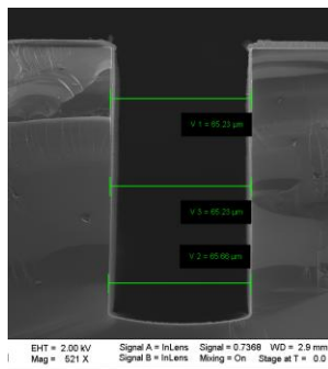
Fig 3. SEM image: cross section of microfluidic channel
