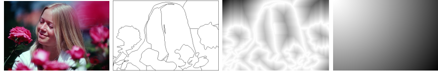
Fig. 7. 239096 Image, One of the Ground truth partitions( G_1 ), Inverse distance function for g_1 , Point ground truth inverse distance function g_p (point at top right), where g_1 and g_p are the corresponding euclidean distance functions
