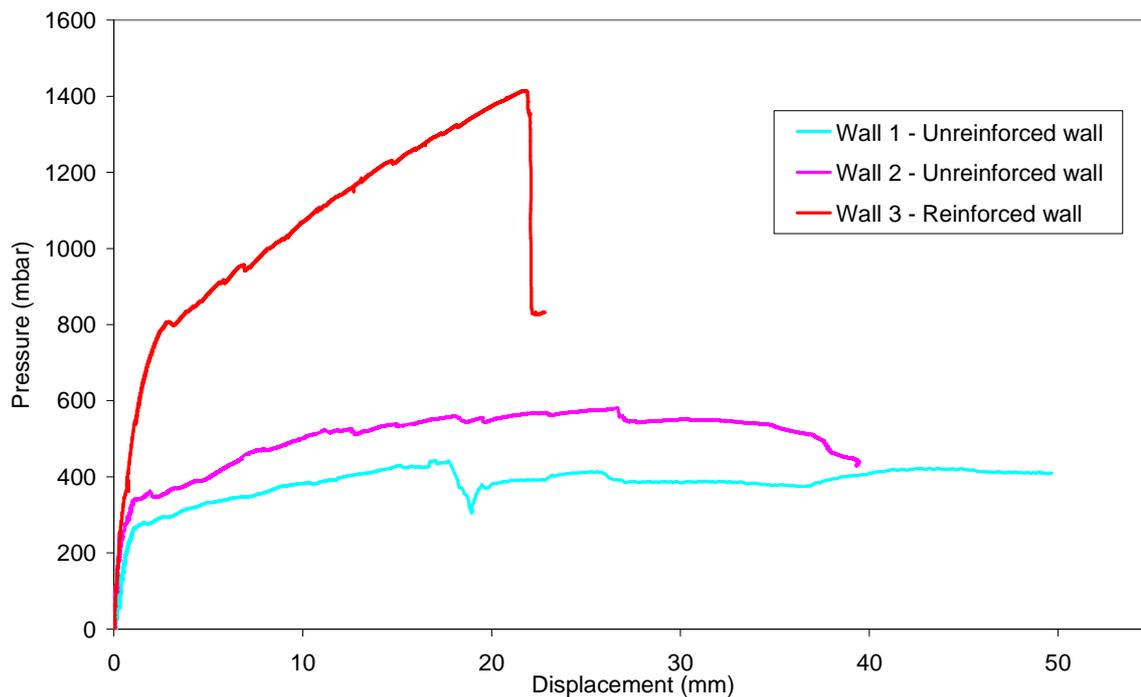
**Figure 7.** Comparison between unreinforced and reinforced wall
