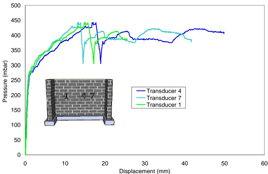
**Figure 4.** Experimental pressure/deflection curve obtained for reference wall
