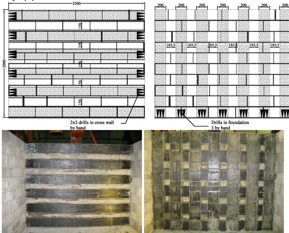
**Figure 6.** Horizontal and vertical reinforcement of the wall
