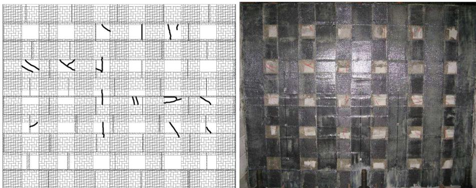
**Figure 11.** Wall 3- Failure mode of the principal wall (0.01mm average thickness of the cracks)
