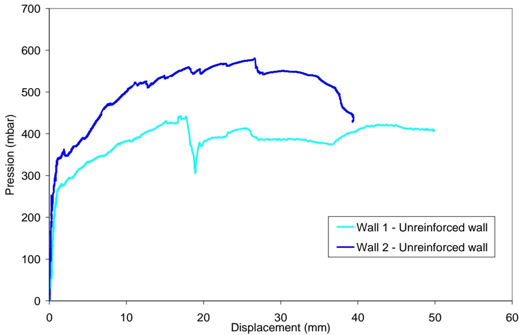
**Figure 5.** Comparison between two unreinforced walls
