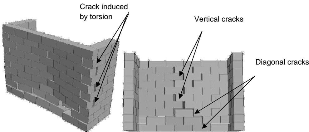
**Figure 14.** The cracking pattern obtained numerically
