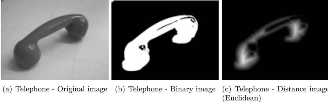
Figure 2.1: A 2D example for distance transformation.
