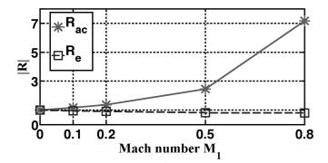
**FIGURE 2**. MODULUS OF THE REFLECTION COEFFICIENT AS A FUNCTION OF INLET MACH NUMBER  $M_1$ . STAR SYMBOL: ACOUSTICAL FORMULATION. SQUARE SYMBOL: ENERGETICAL FORMULATION.
