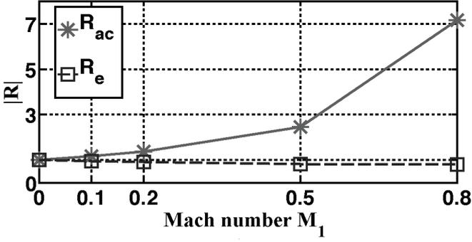
**FIGURE 2.** MODULUS OF THE REFLECTION COEFFICIENT AS A FUNCTION OF INLET MACH NUMBER  $M_1$ . STAR SYMBOL: ACOUSTICAL FORMULATION. SQUARE SYMBOL: ENERGETICAL FORMULATION.
