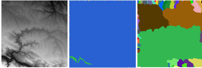
Fig. 61. The gray tone image represents a digital elevation map. The central image shows all regional minima touching the boundary of the image. The right image presents the catchment basins.
