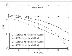
**Figure 7** SFSM MIMO (semi-blind receiver) versus SSSMA (perfect channel knowledge).
