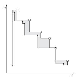
Figure 7: Illustration of the hypervolume difference quality indicator  $(I_H^-)$ . The reference set is represented by boxes  $(\Box)$ , the Pareto front approximation by bullets  $(\bullet)$  and the reference point  $z^I$  by a cross  $(\times)$ . The shaded area represents the hypervolume difference  $I_H^-(\bullet,\Box)$ .
