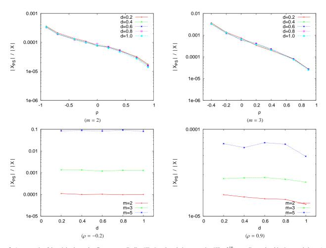
Figure 3: Average ratio of the minimal complete Pareto set cardinality ( $|X_{PS}|$ ) to the solution space size ( $|X|=2^{18}$ ) according to the objective correlation  $\rho$  (top left m=2, right m=3), and according to the Q-matrix density d (bottom left  $\rho=-0.2$ , right  $\rho=0.9$ ). The problem size is n=18. Notice the log-scale.
