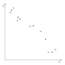
Figure 6: Illustration of the Pareto dominance relation over Pareto front approximations: (i) the approximation ( $\bullet$ ) dominates the approximation ( $\times$ ), (ii) the approximations ( $\bullet$ ) and ( $\circ$ ) are incomparable, and (iii) the approximations ( $\times$ ) and ( $\circ$ ) are incomparable.
