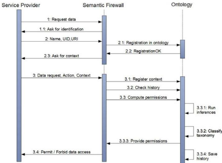
**Fig. 2.** Sequence diagram of the semantic firewall
