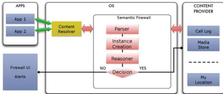
**Fig. 5.** Android porting of the semantic firewall
