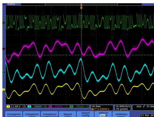
Figure 6. Experimental real-time correction of an arbitrary target movement corrupted by a different arbitrary movement acting on the SSA-SM sensor: (green) SM signal, (purple) corrupted movement, (blue) corrected movement, and (yellow) reference sensor movement.
