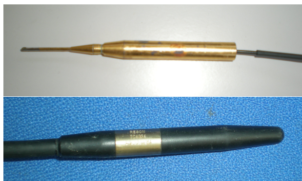
Figure 3: The two hydrophones used : Precision Acoustics PVDF ultrasonic SN 950 (top) and Reson TC4034 (bottom).
