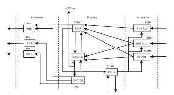
Figure 1. The Flight Application Software
