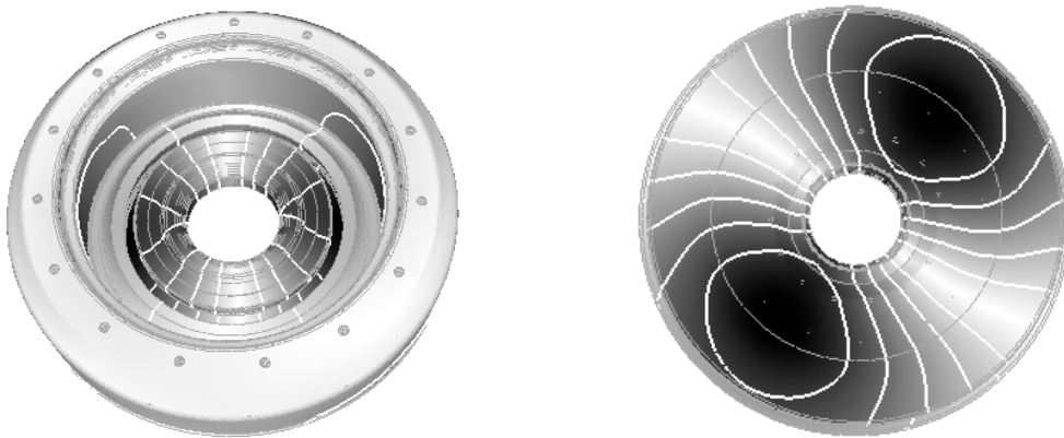
Fig. 25 Field of |\hat{p}| for the 2A mode. View of both sides of the chamber.
