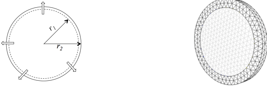
Fig. 4 Academic configuration: cylinder of radius r_2 , with a perforated plate at r_1 , view of the mesh.
