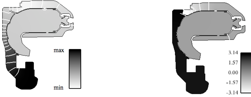
Fig. 20 Field of |\hat{p}| (left) and Arg(\hat{p}) (right) for the 1L mode, U = U_{md} .
