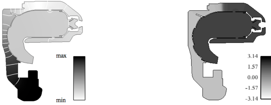
Fig. 17 Field of |\hat{p}| (left) and Arg(\hat{p}) (right) for the 1L mode without plate MP2.
