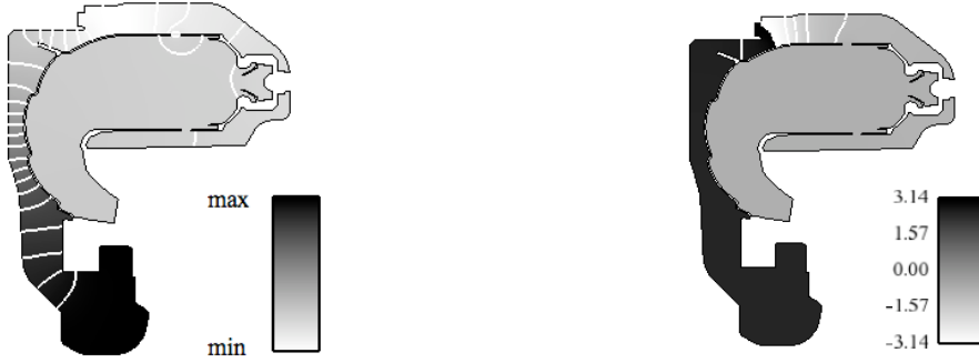
Fig. 21 Field of |\hat{p}| (left) and Arg(\hat{p}) (right), U = U_{md} , without MP2
