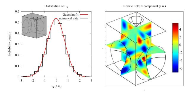
Figure 5: Left: Probability density of the x-component of the electric field for the  $230^{\rm th}$  mode at 1.03 GHz of the cavity shown in insert (Gaussian fit in red). Right: color map of the same component in three orthogonal plane. The results for the other components are similar.
