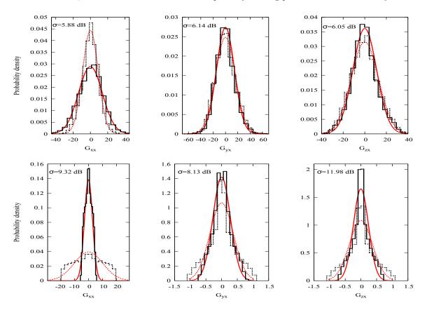
Figure 6: Spatial distribution of the responses for an excitation polarized along the x-axis at a frequency  $f_0 = 953.6$  MHz: in the parallelepipedic cavity (bottom); in the chaotic cavity shown in Fig. 5 (top). All numerical distributions are fitted by a Gaussian distribution (in red). Continuous lines are used for the real part and dotted lines for the imaginary part. The standard deviations  $\sigma$  (in dB) of the power density (see text) are given as inserts.
