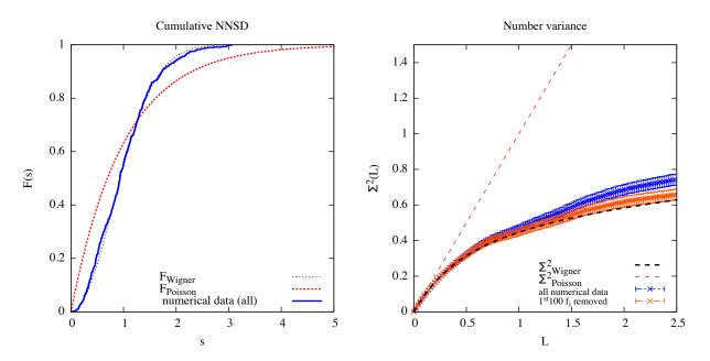
Figure 4: Cumulative NNSD and number variance for the first 571 modes of the cavity with 1 half-sphere and 2 caps shown in Fig. 5. The results obtained are very close to those expected for a chaotic cavity in the universal regime.
