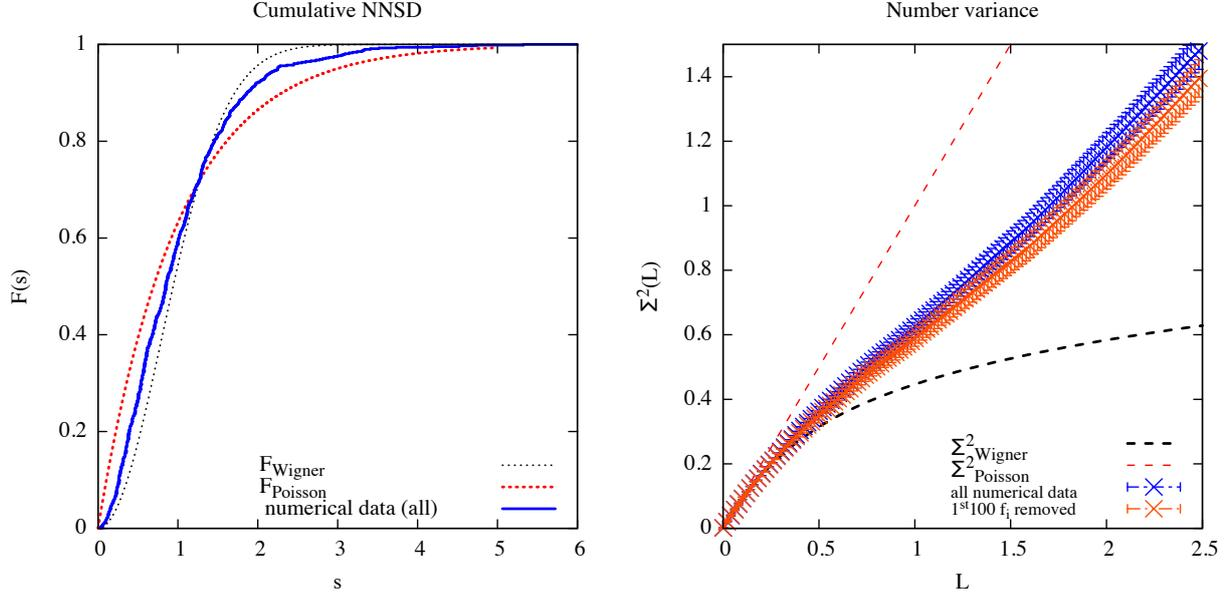
Figure 2: Left: Cumulative distribution function  $F(s)$  for the first 681 modes of the cavity shown in Fig. 1. The numerical data lies between the cumulative distributions associated to  $P_{\text{Poisson}}$  and  $P_{\text{Wigner}}$ . By fitting with  $P_{\text{Weibull}}$  one gets  $\beta = 1.45$ . Right: Number variance for the same data. Even by omitting the first hundred modes (orange data) the agreement with  $\Sigma_{\text{Wigner}}^2$  is barely improved.
