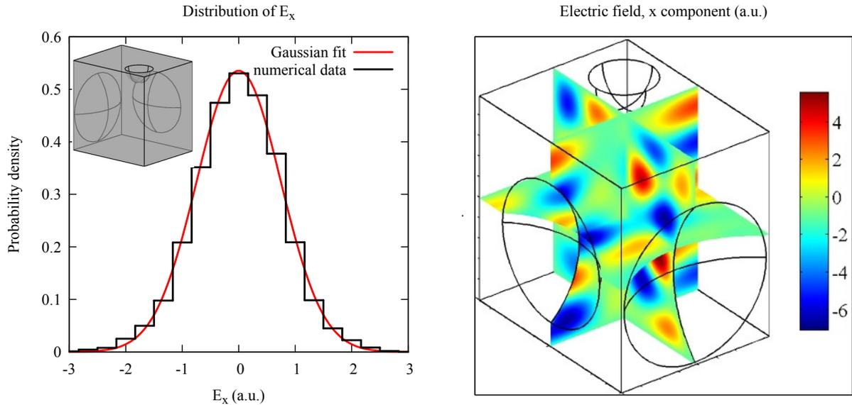
Figure 5: Left: Probability density of the  $x$ -component of the electric field for the 230<sup>th</sup> mode at 1.03 GHz of the cavity shown in insert (Gaussian fit in red). Right: color map of the same component in three orthogonal plane. The results for the other components are similar.
