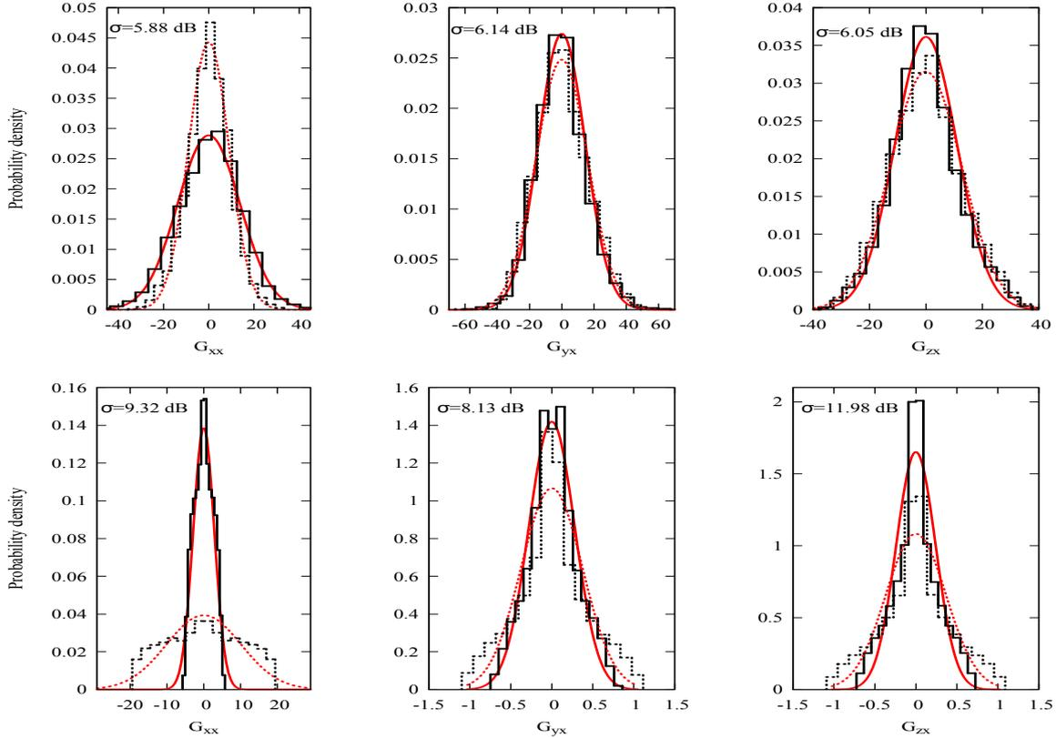
Figure 6: Spatial distribution of the responses for an excitation polarized along the  $x$ -axis at a frequency  $f_0 = 953.6$  MHz: in the parallelepipedic cavity (bottom); in the chaotic cavity shown in Fig. 5 (top). All numerical distributions are fitted by a Gaussian distribution (in red). Continuous lines are used for the real part and dotted lines for the imaginary part. The standard deviations  $\sigma$  (in dB) of the power density (see text) are given as inserts.
