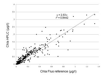
**Figure 3.** Relationship between the chl *a* concentration provided by the reference fluorometer and the chl *a* concentration estimated from HPLC measurements. This relationship was estimated over 70 test profiles ranging between 30 to 200 m and performed between 2002 and 2009.
