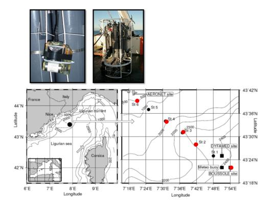
**Figure 1.** Top: CTD-FLUO-SRDL were fixed on the external part of the CTD-cage. Bottom: the Boussole at-sea test set up. Fluorescence profiles were conducted on stations located on the transect between Villefranche sur mer and the BOUSSOLE site (right). A fluorescence profile combined with water sampling for HLPC assessment of Chlorophyll *a* concentration was performed at the BOUSSOLE site located 70 miles off Villefranche sur mer (left).
