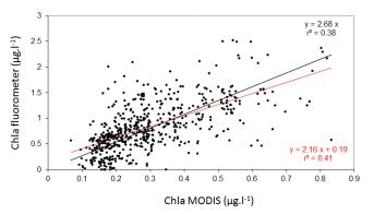
**Figure 9.** Relationship between the offset, quenching corrected HPLC inter-calibrated fluorometers with the corresponding 9 km weekly MODIS data. Both regressions with (in red) and without (in black) intercept are presented.
