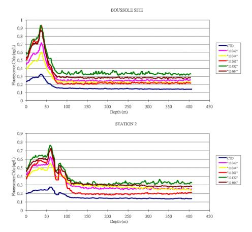
Figure 2. Example of fluorescence profiles provided by different CTD-FLUO-SRDLs and the reference fluorometer (in blue) obtained at two different stations. These profiles exhibit the existence of a fluorescence offset differing between CTD-FLUO-SRDLs. Fluorometers were providing consistent data between each other, but differed in the absolute amount of fluorescence produced.
