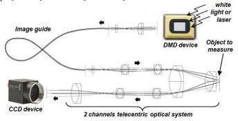
FIGURE 1 - Optical system description
