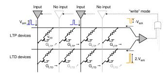
**Fig.13** Write circuit scheme based on the simple STDP rule. For a specific PCM, G  $\nearrow$  denotes an increase while G  $\rightarrow$  denotes no change in conductance.
