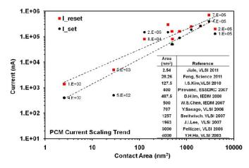
Fig.17 Scaling trend of Reset and Set current for different PCM technologies. Set current values are extracted from literature. Interpolations are also shown
