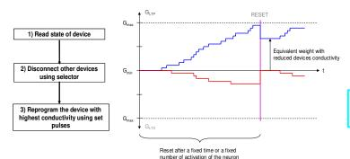
Fig.15 Left: Reset methodology. Right: Conductance G variation of PCM devices before and after a reset sequence.
