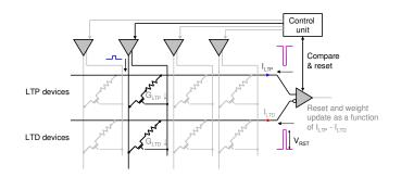
**Fig.14** Reset circuit scheme. For a specific PCM resistor,  $G \downarrow$  denotes a decrease in conductance.
