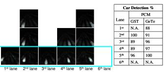
**Fig.16** *Left*: Cars detection for the 6 different lanes by the  $2^{nd}$  layer 10 output neurons. Each block shows the sensitive map of one output neuron. Up to down the detection rate increases. Lane 2 and 5 are learnt by 3 neurons each, while lane 6 is not learnt by any neuron. *Right:* Detection % of 5 best neurons for each lane.
