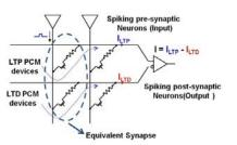
Fig.8 Circuit schematic of the "2-PCM synapse".
