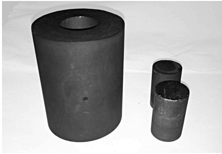
Fig. 1 The graphite die used to bond the copper rods, with the two 20 mm-diameter pressing cylinders
