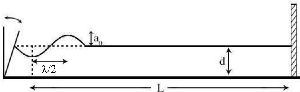
Figure 1. A schematic view of the numerical experiments. Here L is the length of the computational domain, d is the uniform water depth, a_0 is the incoming wave amplitude and \lambda is its wavelength.
