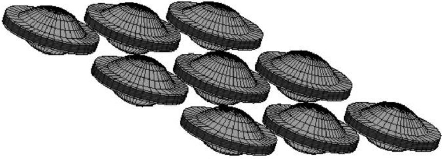
2.21 Deformed mesh of the cymbal array.
