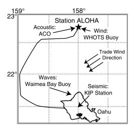
**Figure 2.** Instrumentation map. Data used in this study include ocean floor acoustic data from the ALOHA Cabled Observatory (ACO) at Station ALOHA, wind speed from the WHOTS buoy at Station ALOHA, wave spectra from the Waimea Bay Buoy, and vertical seismic data from the KIP seismic station on Oahu, Hawaii.
