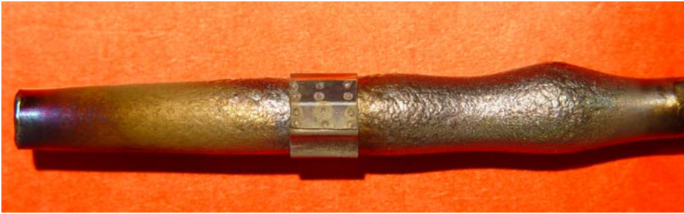
Fig. 4. View of sample with secondary ballooning away from the position of the spacer grid
