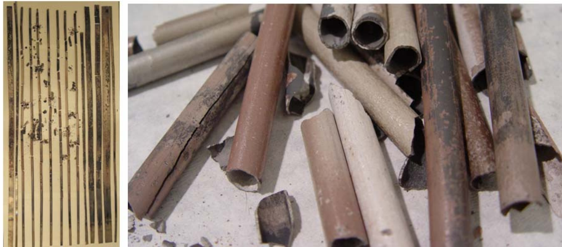
Fig. 12. View of Zr cladding and shroud after seven hours of high temperature oxidation and final quenching by cold water in the preliminary test (left picture: reconstructed vertical state of plates and tubes, right picture: close view of the tubes)
