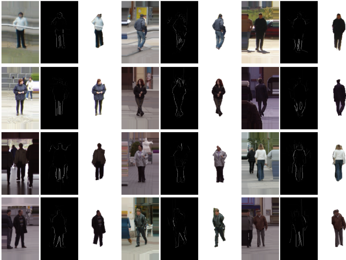
Figure 5: Segmentation of 12 pedestrians in cluttered scenes. From left to right: initial detection window, likelihood of contour segments as being a part of a human silhouette and segmentation obtained with the iterative process.
