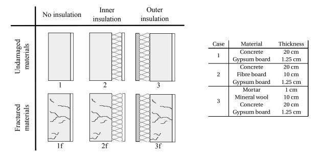
Figure 7: Definition of the simulation cases and materials
