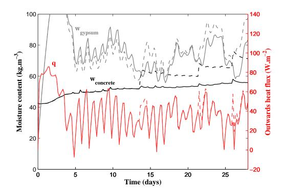
Figure 11: Non-insulated wall (february). Continuous lines: initial wall; dotted lines: fractured wall The interpretation of Fig. 11 leads to the following observations:
