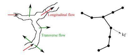
Figure 5: Fracture discretisation and expression of the longitudinal and transverse flow
