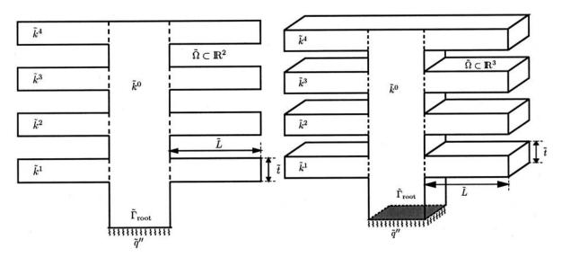
Fig. 1 Two- and three-dimensional thermal fins
