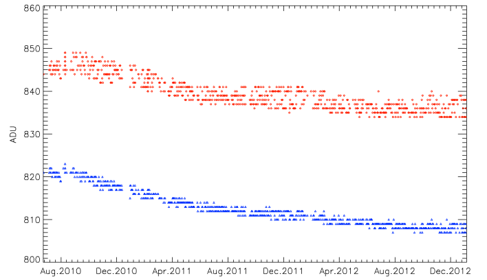
Fig. B.3. Temporal evolution of the offsets of the left port (red diamonds) and right port (blue triangles) of SODISM CCD from July 2010 to December 2012. The offset value is higher and the spread is broader for the upper time series, which corresponds to the left port.
