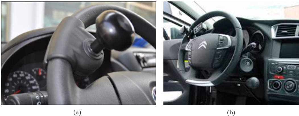
Figure 1: Examples of (a) ball mounted on the steering wheel for total/partial invalidity; (b) radio command used to show the visibility of the vehicle.
