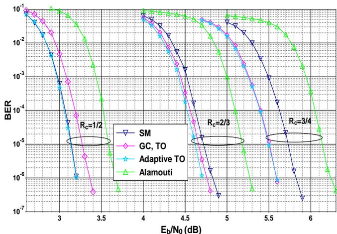
Fig. 6. BER of turbo coded MIMO system; 8-state double binary TC ( $R_c = 1/2, 2/3, 3/4$ ) with 15 turbo-decoding iterations; MIMO profiles: SM, GC&TO, adaptive TO with 4-QAM and Alamouti with 16-QAM; quasi-static Rayleigh fading MIMO channel.
