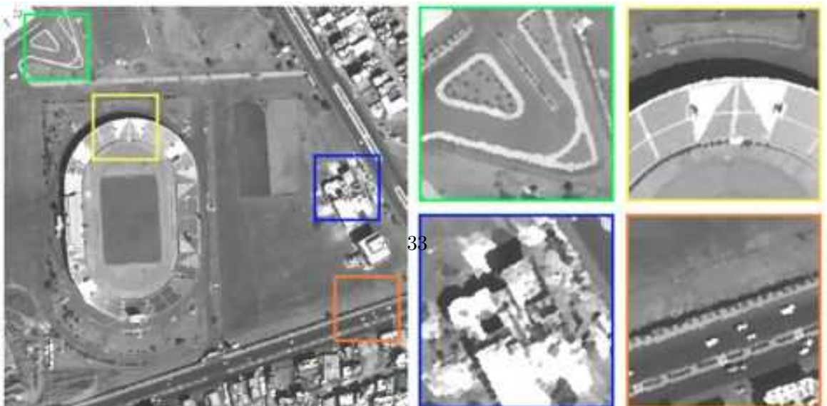
(b) Toggle Mapping ( \tau_{SE}^{\infty}(\mathbf{I}) ) of (a). Computational time is 9.95 sec.
