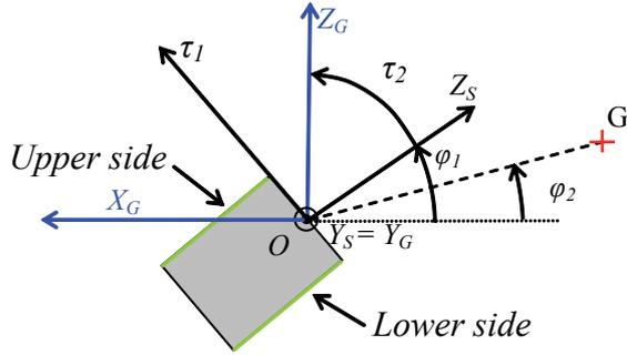
1: Description of the section geometry.  $O(X_s, Y_s, Z_s)$  is the reference system corresponding to a given section, with  $Z_s$  equal to the local pith orientation  $n$ ;  $O(X_G, Y_G, Z_G)$  is the reference system corresponding to the tree;  $O$ : biological centre of the section;  $G$ : centre of mass of the upper part of the tree;  $\varphi_1$ : tilt angle of the section;  $\varphi_2$ : tilt angle of the tree.
