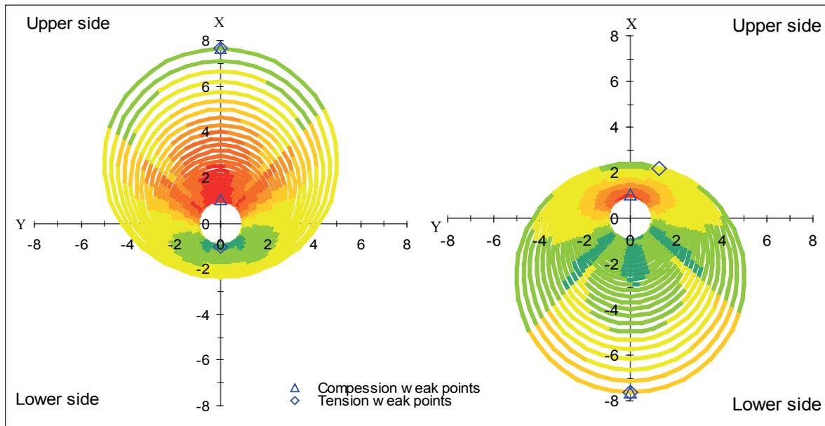
4: stress distribution and location of weak points in a hardwood (left) and in a softwood (right): section exhibits an important eccentricity ( $e = \pm 2/3$ ) with occurrence of juvenile and reaction wood; red areas represent maximal compressive stresses, green areas maximal tensile stresses
