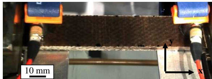
Figure 4. View of hemp/epoxy composite specimen with AE captors placed on it.
