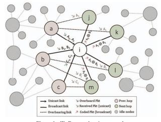
Figure 1 - ZigBee overhearing example
