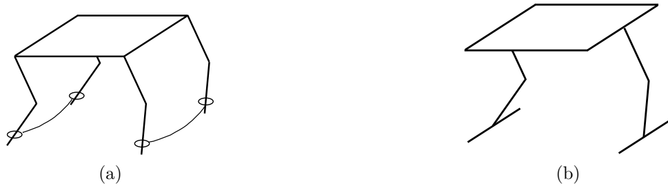
Figure 1. (a) Quadruped with coupled front and coupled back legs, (b) Quadruped with two virtual legs.
