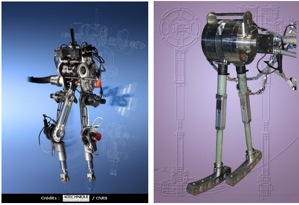
Fig. 1. Biped bipeds, “Rabbit” (left) and “Emu” (right).
