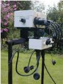
Figure 14 : Resistivimeter "RM-15" and multiplexer "MPX-15".
