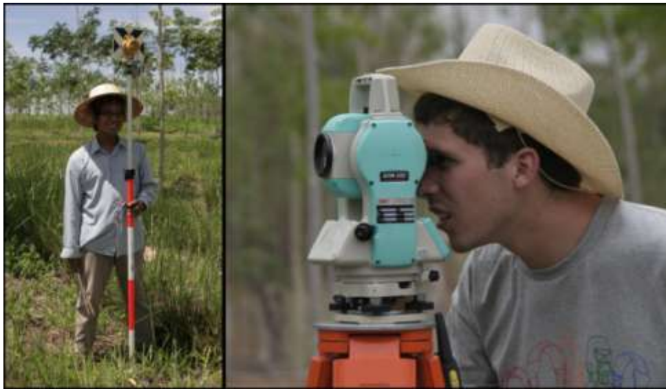
Figure 7 : Topographic measurements with the Total Station Nikon DTM-332.
