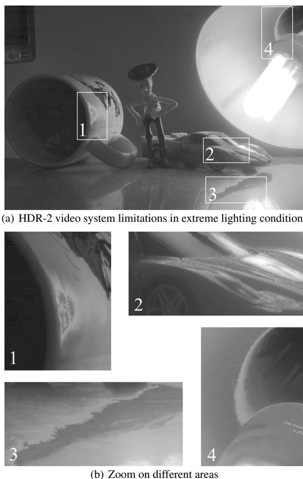
**Fig. 11** HDR-2 system limitations in extreme light conditions.
