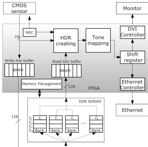
Fig. 2 Overview of the HDR-P video system architecture.
