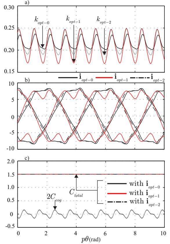
Fig. 12. Control performance with a cogging torque; a)  $k_{opt-0}$ ,  $k_{opt-1}$  and  $k_{opt-2}$  (A/Wb) obtained by the Adaline controller; b) optimal currents obtained with three approaches (A); c) torque developed (N.m) and cogging torque (N.m)
