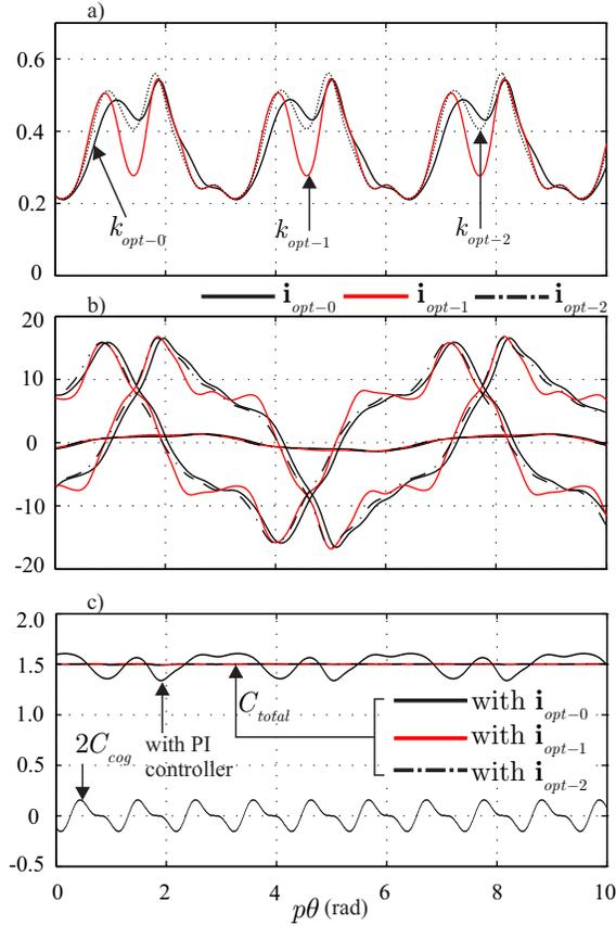
Fig. 13. Control performance with a cogging torque and a fault on one phase; a)  $k_{opt-0}$ ,  $k_{opt-1}$  and  $k_{opt-2}$  (A/Wb) obtained by the Adaline controller; b) optimal currents obtained with three approaches (A); c) torque developed (N.m) and cogging torque (N.m)
