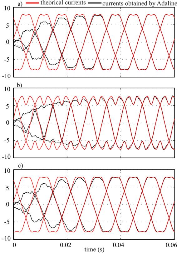
Fig. 10. a)  $i_{opt-0}$  obtained with (41) learned by an Adaline ; b)  $i_{opt-1}$  obtained with (42) learned by an Adaline; c)  $i_{opt-2}$  obtained with (43) learned by an Adaline ( $\Omega = 314\text{rad/s}$  and  $\eta = 0.1$ )
