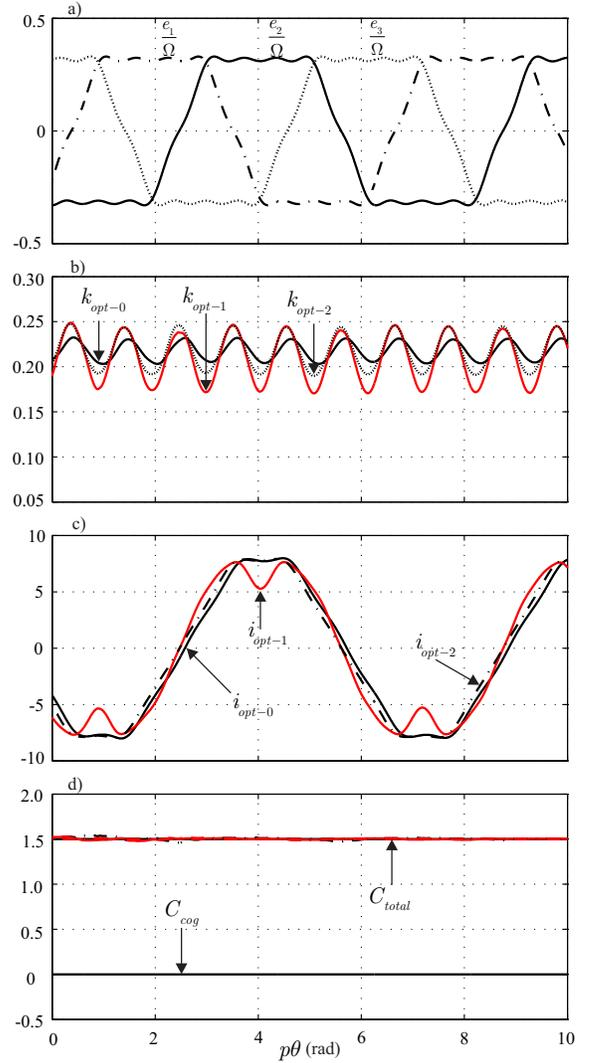
Fig. 8. Simulation results of a three-phase non-sinusoidal machine: a)  $\Phi'_1, \Phi'_2, \Phi'_3$  (Wb); b)  $k_{opt-0}, k_{opt-1}$  and  $k_{opt-2}$  (A/Wb) obtained by the Adaline controller; c) optimal currents (one phase) obtained with three approaches (A); d) torque developed (N.m)
