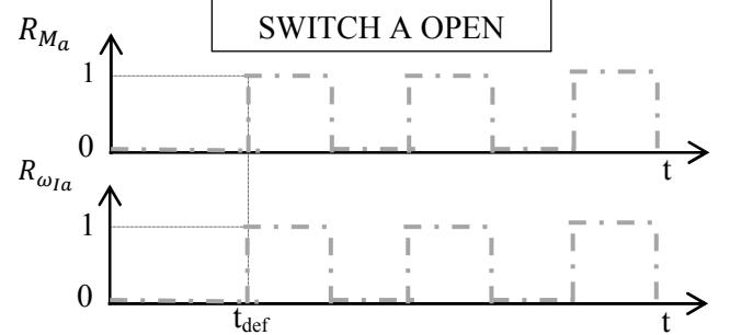
Fig. 10. Theoretical values of the fault indices in case of open-switch fault occurring at time  $t_{def}$ .
