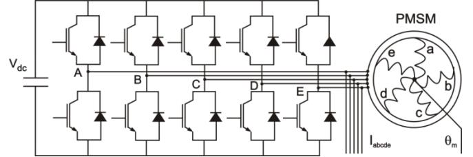
Fig. 1. Drive topology composed of a single energy source, a five-leg inverter and a five-phase star-connected PMSM.
