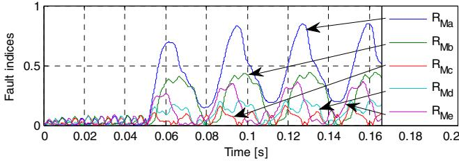
Fig. 7. Magnitude indices in case of open-switch fault occurring at time  $t=0.05\text{s}$  (top switch of phase  $a$ ).
