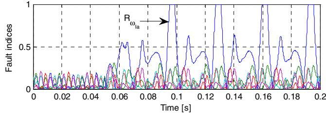
Fig. 8. Frequency indices in case of open-switch fault occurring at time  $t=0.05\text{s}$  (top switch of phase  $a$ ).
