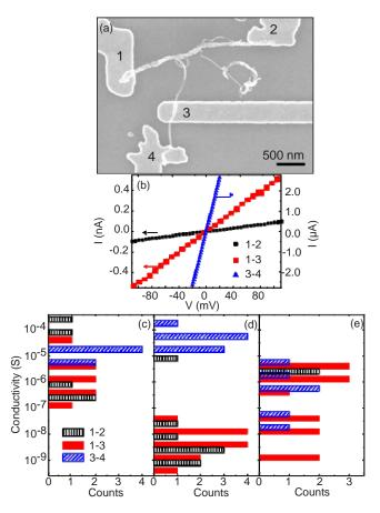
FIG. 2. (Color online) (a) SEM image and (b) *I-V* characteristics of an electrically connected CNT junction obtained from MWNT-FeO<sub>x</sub>NP conjugates. [(c)–(e)] Histograms of conductances (see Ref. 20) for (c) MWNT-ferritin, (d) MWNT-FeO<sub>x</sub>NP conjugate, and (e) DEP deposited MWNT and FeO<sub>x</sub>NP samples. The primary CNT is measured between electrodes 1 and 2, the secondary CNT between 3 and 4 and the junction between 2 and 3.
