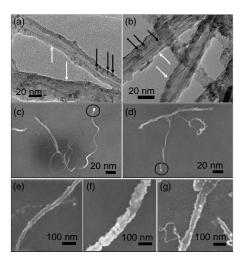
FIG. 1. TEM images of (a) MWNT-ferritin and (b) MWNT-FeO<sub>x</sub>NP conjugates, showing CNTs (white arrows) decorated with metal particles (black arrows). SEM images of individual regrowth events from (c) MWNT-ferritin and (d) MWNT-FeO<sub>x</sub>NP conjugates. Circles show the probable location of the catalyst particle. SEM images showing the primary MWNTs after CVD growth in (e) MWNT-ferritin, (f) MWNT-FeO<sub>x</sub>NP, and (g) MWNT with DEP deposited FeO<sub>x</sub>NP samples.
