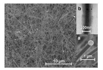
Fig. 1 SEM observations of SiNWs film obtained at 550 °C. a Zoom on a gold droplet in. b TEM observation of a silicon nanowire after a first reduction down to 20 mV
