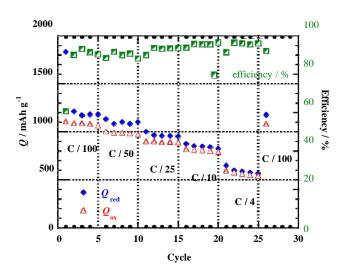
Fig. 4 Influence of the rate capability and coulombic efficiency as a function of the cycle number for SiNWs film grown at 540 °C during 15 min
