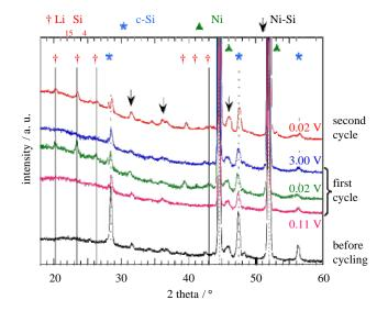
Fig. 5 XRD patterns of SiNWs films, grown at 540 °C during 15 min, before electrochemical cycling, during the first cycle when material is discharged to 0.11 V and 0.02 V and charged up to 3.00 V, and when fully discharged to 0.02 V during the second cycle (70  $\mu$ A cm<sup>-2</sup>)
