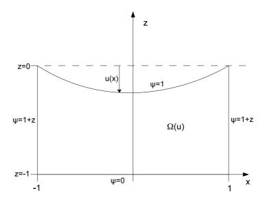
FIGURE 1. Idealized electrostatic MEMS device.
