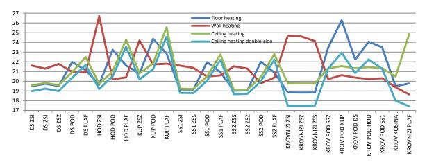
Figure 8 The mean temperatures of surroundings walls, floors and ceilings during January
