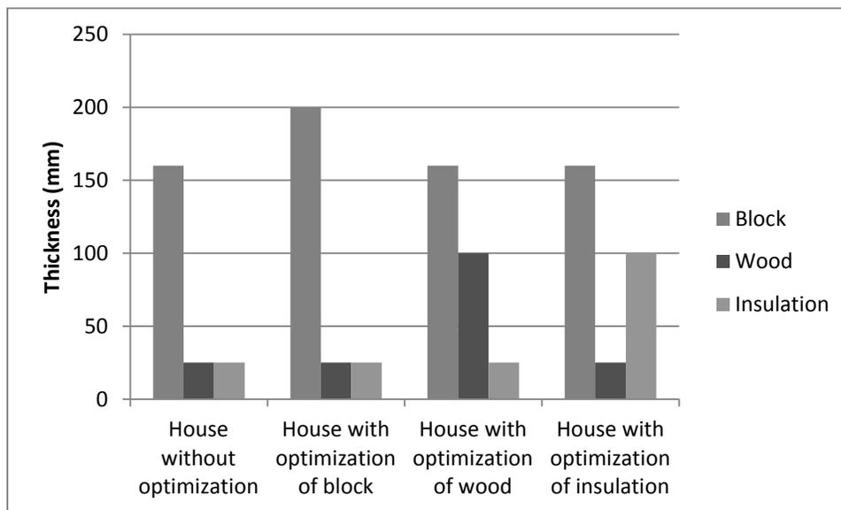
Fig.4: Thickness of the wall layers for a house with optimizations and without optimization
