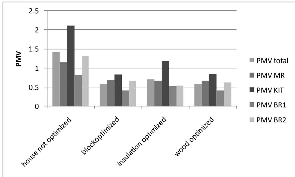
Fig.3: Comparison of PMV between house no optimized and house with different layer optimized
