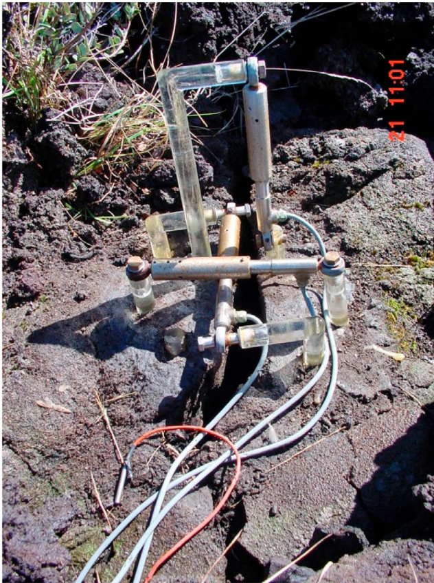
Figure 3. FORx extensometer located at the base of the summit crater of Piton de la Fournaise. The length of the crack is about 10 m and the opening of the crack is around 2 cm.
