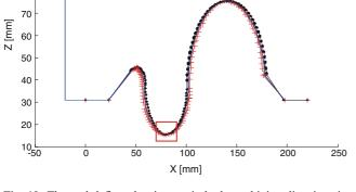
Fig. 19 The tool deflected trajectory in both machining directions in the plan XZ
