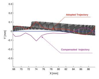
Fig. 21 The tool trajectory compensated
