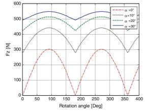
c) The effect of the inclination angle  $\alpha$  upon  $F_z$
