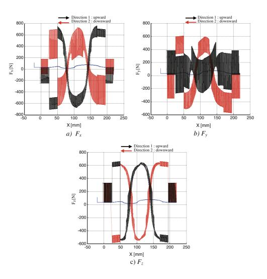
cut. The cutting forces are drawn in black for the X machining, and in red for the -X machining.
