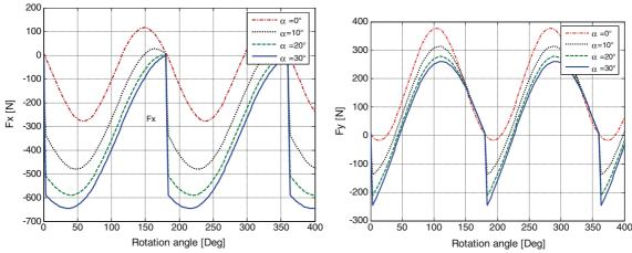
*a)* The effect of the inclination angle  $\alpha$  upon  $F_x$
