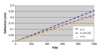
Fig. 8 The evolution of the deflection according to the force F
