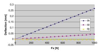
Fig. 10 The tool deformation evolution according to the effort exerted
