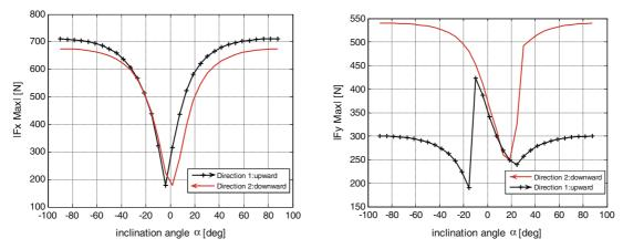
a) The effect of the inclination angle  $\alpha$  upon  $|F_{xmax}|$  b) The effect of the inclination angle  $\alpha$  upon  $|F_{ymax}|$
