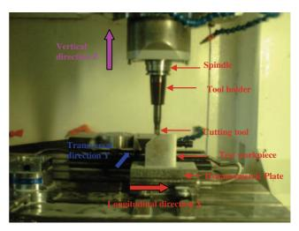
Fig. 11 Tool deflection measuring method on tool machine
