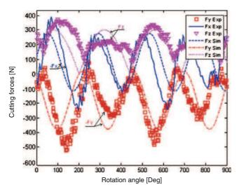
Fig. 4 Simulated and real cutting forces exerted on the dynamometric plate
