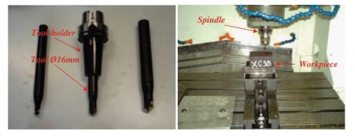
They also allow us to record a difference in amplitude between two consecutive teeth. This gap is due to a problem tool eccentricity according to the spindle axis.
