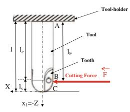
Fig. 7 The loading of the tool
