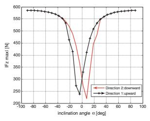
c) The effect of the inclination angle  $\alpha$  upon  $|F_{zmax}|$
