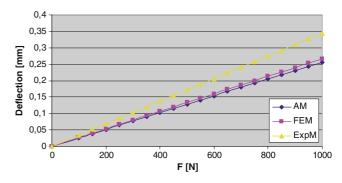
Fig. 13 The deflection evolution, according to the load of the tool, recorded with the three methods: the AM, FEM, and Exp
