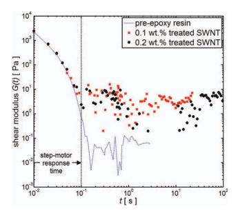
**Figure 1** Shear modulus of an epoxy resin and two different dilute suspensions of treated SWNT within an epoxy resin. Response after a 1% shear-strain step. Isothermal tests at 25°C. Courtesy of Dr. Anson Ma (Rice University). [Color figure can be viewed in the online issue, which is available at wileyonlinelibrary.com.]
