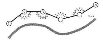
**Figure 2** Nonfreely jointed bead rod chain model composed of n beads and n - 1 rods of length a. Bending potential between rods in the bead rod chain is mimicked with a hypothetical flexion spring. An equivalent continuous semiflexible filament is depicted below the discritized model.
