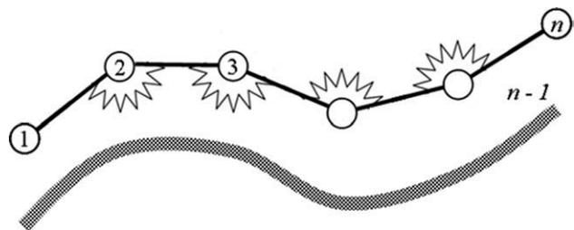
**Figure 2** Nonfreely jointed bead rod chain model composed of  $n$  beads and  $n - 1$  rods of length  $a$ . Bending potential between rods in the bead rod chain is mimicked with a hypothetical flexion spring. An equivalent continuous semiflexible filament is depicted below the discretized model.
