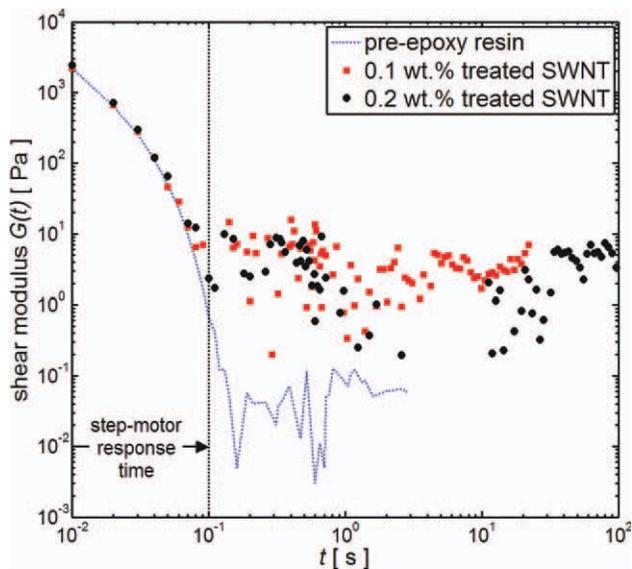
**Figure 1** Shear modulus of an epoxy resin and two different dilute suspensions of treated SWNT within an epoxy resin. Response after a 1% shear-strain step. Isothermal tests at 25°C. Courtesy of Dr. Anson Ma (Rice University). [Color figure can be viewed in the online issue, which is available at [wileyonlinelibrary.com](http://wileyonlinelibrary.com).]
