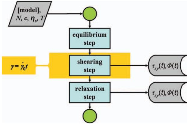
**Figure 3** Flowchart of the general BD algorithm for simulating a shear-strain step test. [Color figure can be viewed in the online issue, which is available at [wileyonlinelibrary.com](http://wileyonlinelibrary.com).]
